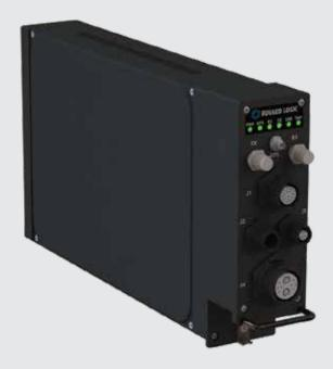
At the core of the AXIOM AIR is the Teledyne Paradise Datacom AXIOM-X modem. This compact, yet powerful, DVB-S2X modem provides broadband connectivity while being extremely bandwidth efficient. Additionally, the compatibility of the AXIOM-X with other Paradise modems gives users the ability to extend their networks into new and smaller aircraft.
